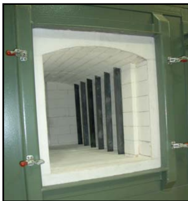
Insulating Fire Brick (IFB) Lining
