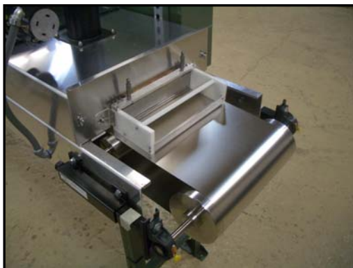
TC-101SLC/SMLC feature a stainless steel belt
