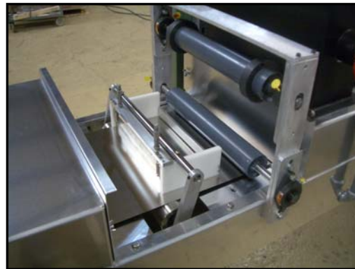
LabCast with tandem doctor blade and interleaf dispenser
