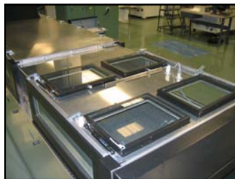
Casting Area Access Windows
