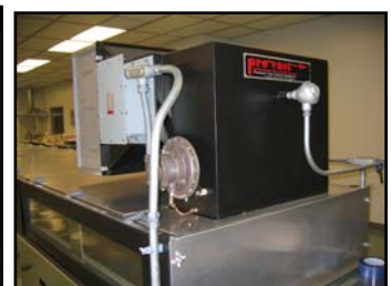
Process Air Heater
