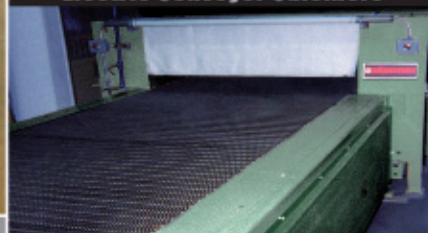
Electric Conveyor Calciners
